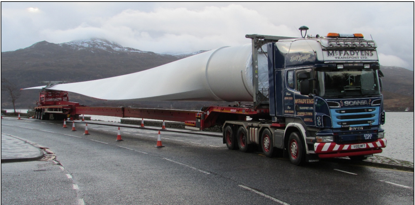
Figure 2-2: Superwing Carrier Trailer
